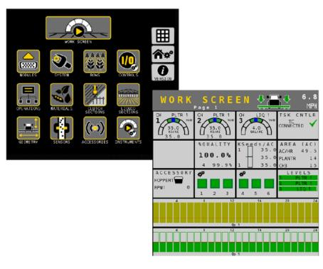
The ISO6 Intelliag system is the latest ISOBUS Rate Controller from Dickey-john. The system supports up to 48 rows of Individual Row Control, ensuring accurate seeding rates across the entire bar, even while turning, using Row by Row Turn Compensation.
