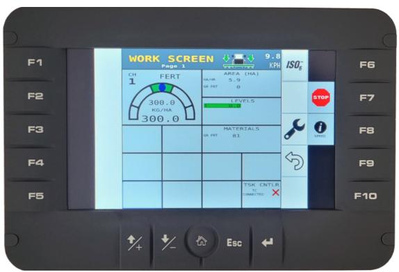
The TERA 7 Universal Terminal is the 7" touchscreen display by Cobo. The Terminal is ISOBUS-compatible and comes with all tractor harnessing, making it the perfect standalone display for basic rate-control and monitoring applications.
